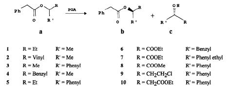
Scheme 1: Mode of hydrolysis of phenylacetyl esters of secondary alcohols
